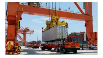
The solution LaseTPC - Truck Positioning Crane is designed to take over a fully automated truck positioning under STS cranes. The use of robust and state-of-the-art laser technology has the aim to reduce personnel in such danger zones while STS spreader operations.
