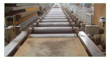
A continuous monitoring of slabs on a cold roller table is possible with the LaseSTR – Slab Tracking Roller-table measurement system.
