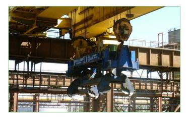
The application LaseSPY – Slab Positioning Yard for an automatic slab-yard is used to transport slabs in pick and drop operations without any crane drivers.
