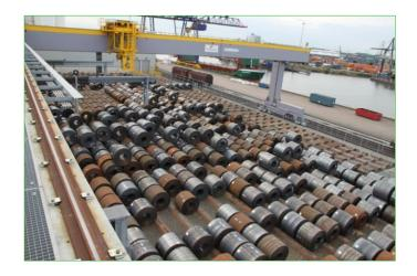
The application LaseCPY – Coil Profiling Yard is used to measure the positions of coils in crane, trolley and height direction.
