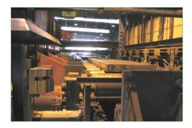
By using the measurement system LaseSPF – Slab Positioning Furnace slabs can precisely be positioned before being pushed into the furnace.
